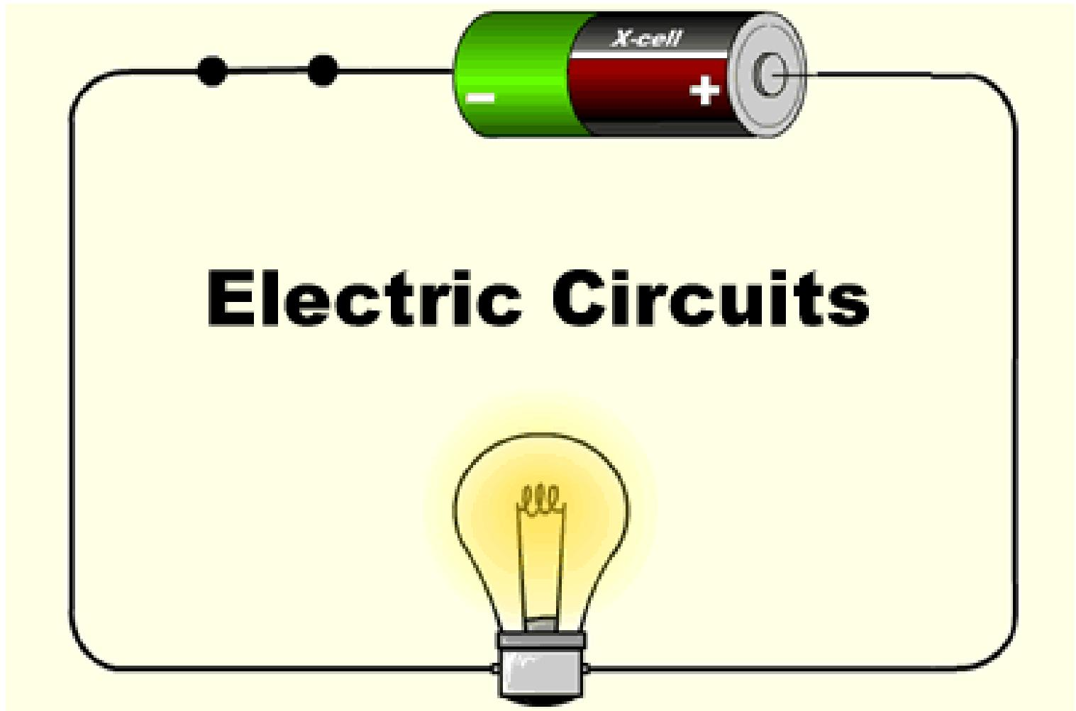
Electricity doesn't flow by itself. It needs a push. A battery can push electricity through a circuit (like a water pump pushing water through a hose).
